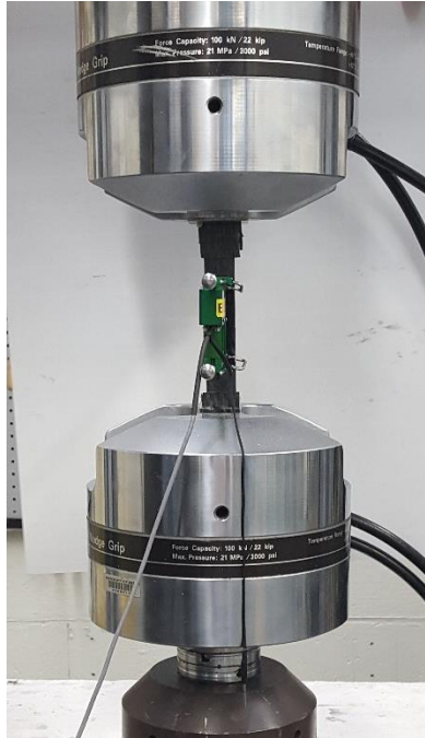
Figure 5.1 - Tensile test set-up
