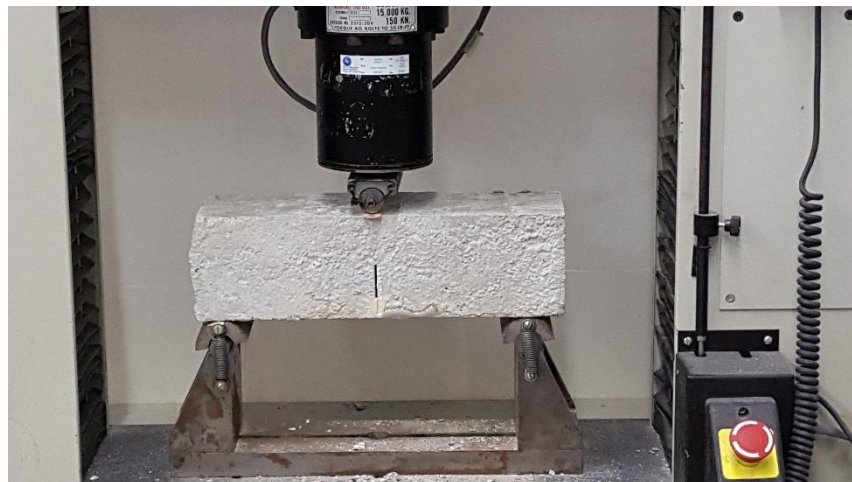
Figure 12.2 – Shear bond test set-up
