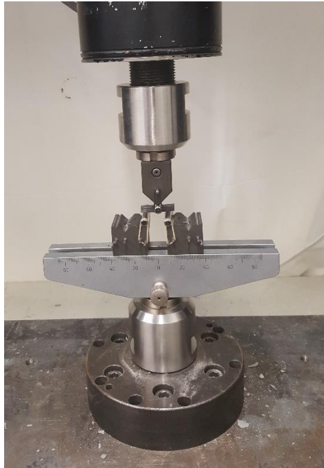
Figure 10.1 – Interlaminar shear test set-up
