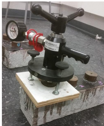
Figure 11.2 – Tension bond strength test set-up
