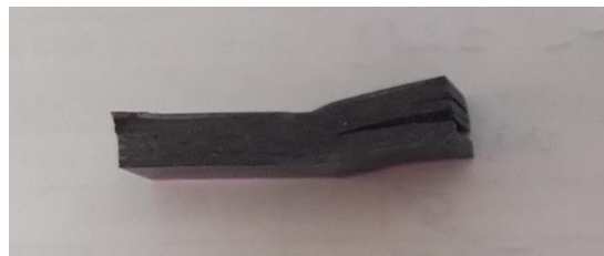
Figure 10.2 – Representative failure mode showing interlaminar shear between plies
